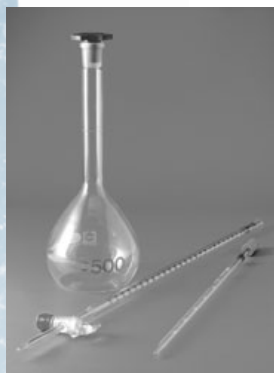
figure 4.10 Preparing solutions of accurate concentration requires the use of precise glassware such as a volumetric flask, a pipette and a burette.
