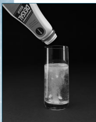
figure 8.2 Effervescence in this antacid preparation is due to hydrogen ions and hydrogen carbonate ions reacting together to produce bubbles of carbon dioxide.
