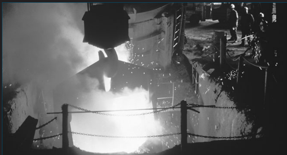
figure 7.1 Extraction of iron in a blast furnace is a redox reaction.
