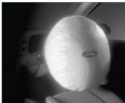
figure 5.2 The air bag in a car makes use of the rapid movement of gas particles produced by a chemical reaction to fill the space of their container.
